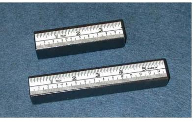
I think once you tried using similar building blocks, you will like them. They do work well on small models. I've built a 1/2A Stardust's wing and tail using the block hold down method instead of pinning the flying surfaces down to a flat building table. I will also use them in the building of Holman's kits Fokker DVIII.
